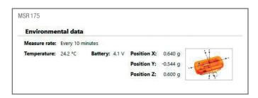
**MSR PC-Software:** In the setup with «Read» on the MSR145 / MSR165 or «Click here to view values» on the MSR175 and MSR175plus, the current values ACCx, ACCy, ACCz can be read.
